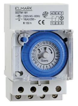
The mechanic relay for time is supposed to be used for managing chains with maximum capacity of 3500W.After the setting, the timer executes the functions we required in 24 hours regime. The minimum period for setting is 30 minutes as it is executed within 48 pcs segments which the timing of the work and rest of the consummator is being set. The timer is accomplished with a battery which assures the work by 150 hours after power failure.
